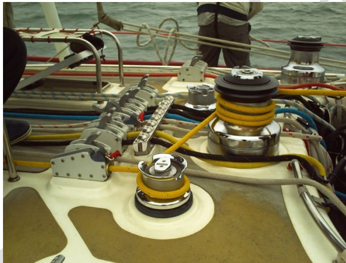
Dolly winch being used with the main halyard.
